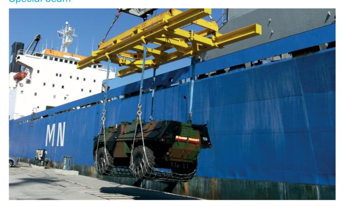
Lifting beam with adjustable lifting points
